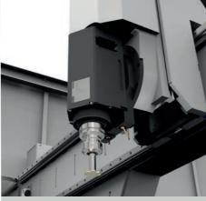
MACHINING HEAD allows machining on 3 sides of the profile and on the 2 ends.
