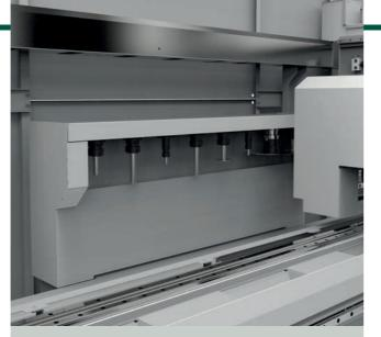
**FIXED TOOL MAGAZINE** on base allowing up to 8 tools to be loaded (optional)
